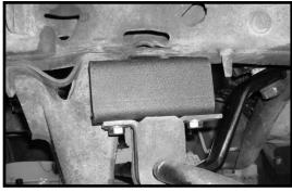
47. Move back to the stock lower sway bar end link mount-∎relocation the to the previously drilled hole using the new ing hardware and add some thread locker or loctite on both 5/16" x 1" bolt and hardware. Make sure to use thread lockthe driver and passenger side and torque to 65 ft lbs.
