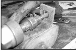
44. Locate the stock sway bar and the stock sway bar lower hardware. Working on the driver side, install the stock sway bar end link into the stock lower location and secure using the stock hardware. **Do not tighten at this point**. Repeat procedure on the passenger side. Let the stock sway bar hang.
