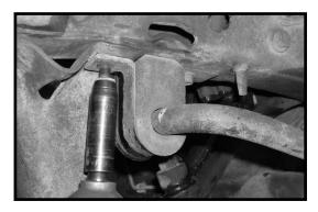
Working on the driver side, remove the stock sway bar carded. end link from the stock axle location. Save the hardware Repeat procedure on the passenger side. Set the sway bar aside.
