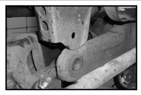
7. Working on the front driver side twin eye beam axle bracket, remove the stock bracket from the stock location. Save the stock hardware but the the stock bracket may be dis-
