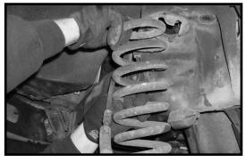
18. Working on the driver side, remove the stock radius arm from the stock location. Save the stock hardware and front sway bar bracket. The stock radius arm may be discarded. Repeat procedure on the passenger side.
