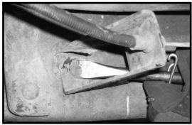
21. Using the 15" mark on the side of the frame rail as a guide and using a straight edge, scribe a mark on the bottom of the frame rail.
