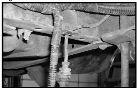
71. Locate the new rear brake line relocation bracket, (1)
