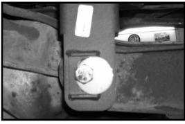
into the newly installed bracket. Secure the axle to the new∣sway bar may need to be opened up to 7/16". Try a 7/16" bolt bracket using the new cam bolt and hardware. Make sure to in each location to make sure that it will fit. If not, open the
