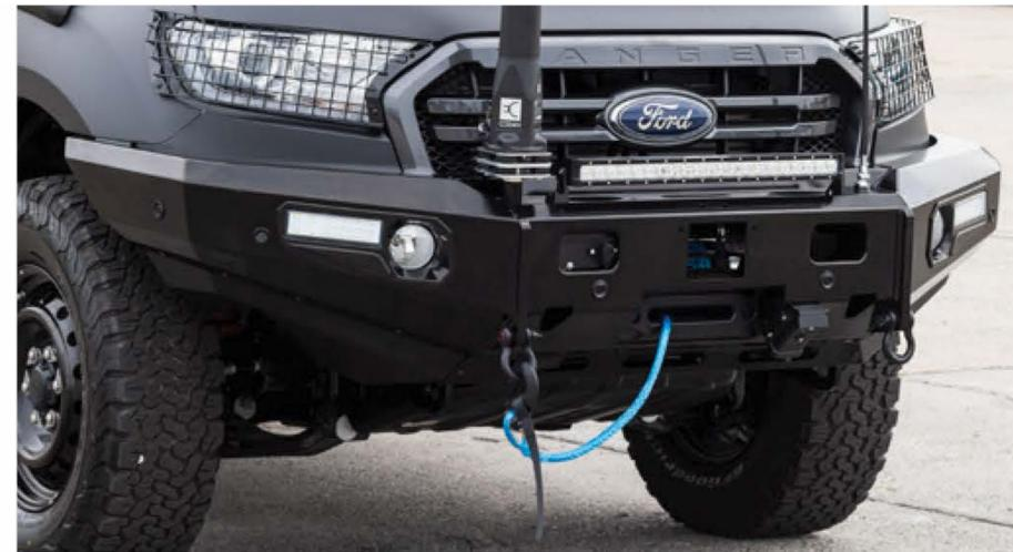
Front bumper with electric winch and LED driving light
