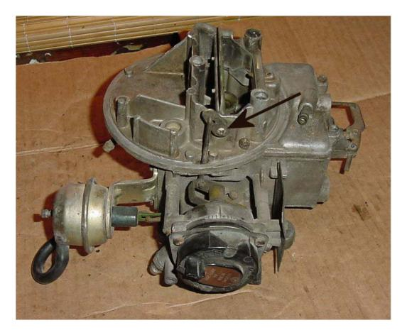
Remove the choke (black plastic piece) by removing the three screws and clamp
