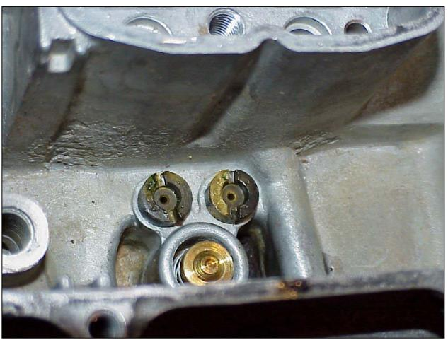
Next put the needle seat in. There should be a gasket between the needle seat and the carb.
