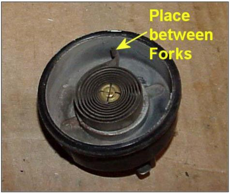
Install the Choke cover clamp but leave loose so you can turn it to adjust.
