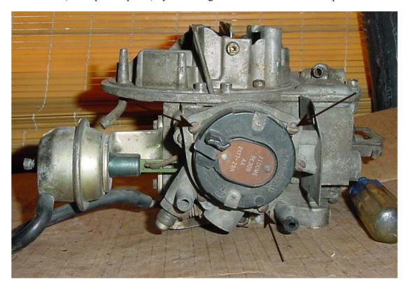
Choke housing removed. The next step is an option, there is a small gasket behind the choke housing. To get to it, you will have to remove the three screws the holds the housing to the carburetor. This can be a big mess when putting back together. I usually don't replace the gasket and leave the housing attached when cleaning the carburetor. Just tighten the three screws after cleaning.
