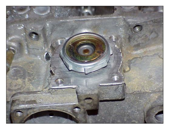
Install new gasket for the power valve cover.
