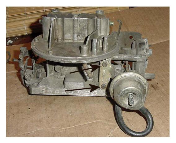
Remove the C-Clip that the choke pull off rod to the choke pull off. Remove the vacuum line and remove the unit from the carburetor.
