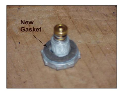
Install power valve into the bottom of the carburetor. The power valve should be on tight but not gorilla tight. You don't want to crush the gasket
