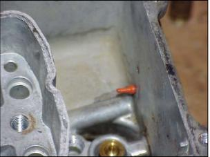
I start on the outside front. For the accelerator pump the first thing you need to do is insert After that comes the return spring and diaphragm. The wide end of the spring should touch the base of the carb and the button on the diaphragm should face outward. Put the cover over the diaphragm and insert the 4 screws.
