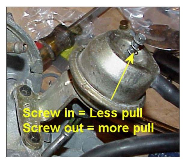
When you put this back on the engine and it idles to high during warm up. You can adjust this screw to raise or lower the RPM.
