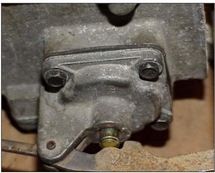
Insert the accelerator pump rod into the proper hole on the pump arm. Attach the other end of the rod to the throttle with the retainer into the third hole.
