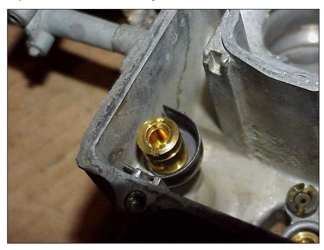
Install the float clip onto the needle.
