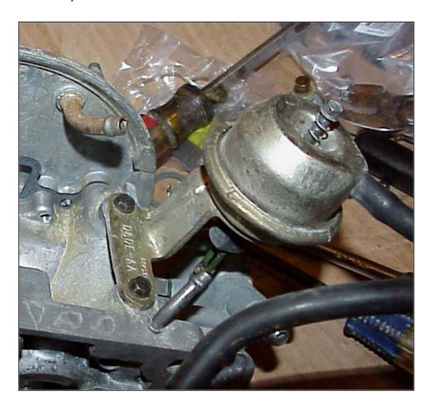
Install the choke cover gasket, choke cover and spring. Be sure that the spring fits between the forks.
