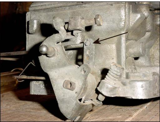
On the front of the carb remove the 4 screws for the accelerator pump. Inside the pump there should be a diaphragm type element and a spring. There is also a rubber plug attached to the base of the carb (remove later).
