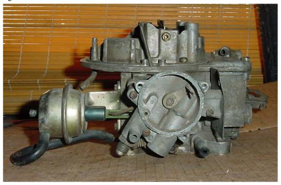
Remove the two screws that holds the choke pull off to the carburetor
