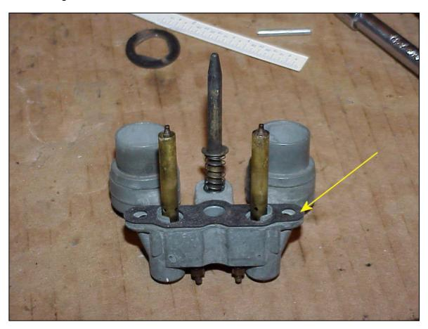
Install the small metal ball into the hole in the middle where the venturi cluster goes.
