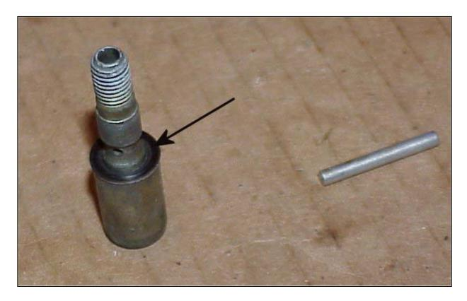
Insert the weight into the hollow screw.
