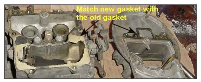
Remove the carb internals starting with the float. The rod that holds the float is secured by the wire clip that runs behind the needle seat. Use a pair of long nose pliers to remove the wire clip and the rod with the float can then be removed.
