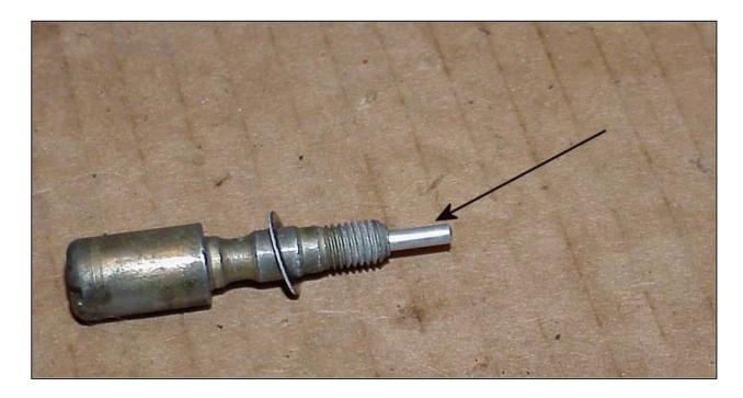
Now very carefully insert the hollow screw into the venturi cluster. You can also insert the weight into the hole first than the hollow screw. You may have to shake things a little to get the screw to drop over the rod.
