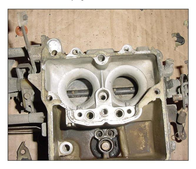
Flip the carburetor over and remove the fuel/air mixture screw. Some people note how many turns it takes to remove them such that they can be put back at the same position when the carburetor is reassembled. I would do this as a backup measure in case there is difficulty setting the idle mixture per the shop manual method. Also remove the 4 screws that hold the power valve cover.
