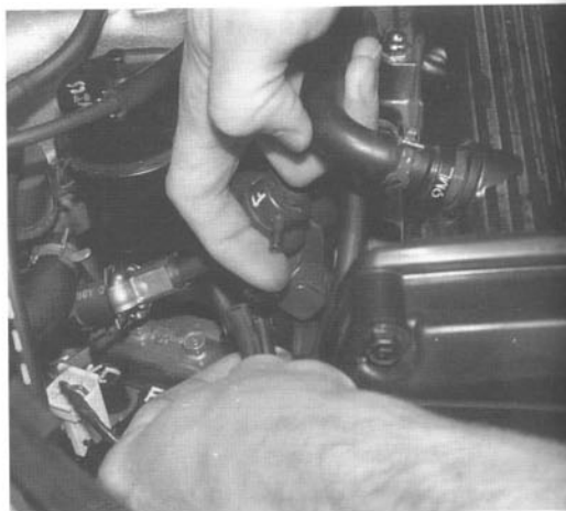
Fig. 2-5. Check for evidence of fuel at regulator vacuum port. If it is dry, the diaphragm is not leaking.
