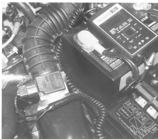
Fig. 4-14. In Continuous Monitor Test (EEC-IV only) you attempt to recreate fault while checking for codes. For example, tap MAF sensor while watching STAR tester.
