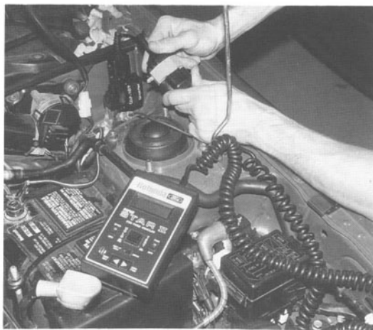
Fig. 4-10. STAR tester hookup to read trouble codes.
