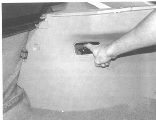
Fig. 2-8. Inertia switch in trunk.
