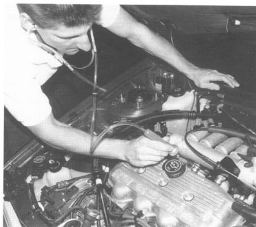
Fig. 2-12. You can check injector operation with a stethoscope or by placing screwdriver tip against injector body and listening for clicking sound.
