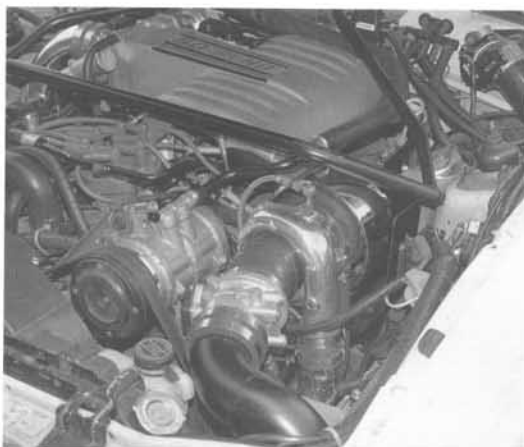
Fig. 6-9. Turbo Technology T04 water-cooled turbo.
