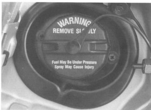
Fig. 2-7. Ford sets relief valve in the fuel tank cap at 1.6 psi (11 kPa). That small pressure can force fuel out of an open return line.
