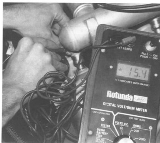
Fig. 2-13. Checking injector resistance.
