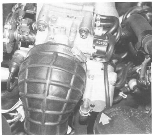
Fig. 4-10. Combination ISC-BPA (arrow) on 1.8L engine.
