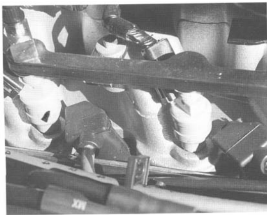
Fig. 2-3. Port injectors are mounted in manifolds at intake ports.
