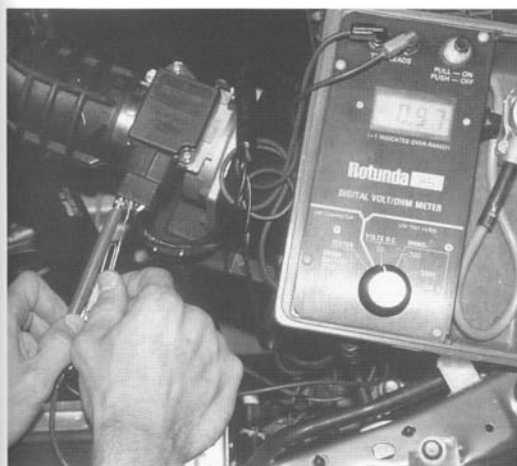
Fig. 3-1. Checking Mass Air Flow (MAF) sensor output with engine running.
