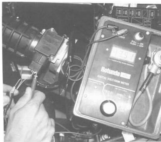
Fig. 1-1. Backprobing gives you access to circuit signals without breakout box. Checking VPR to Mass Air Flow (MAF) sensor shown. Take care not to damage connector or terminals.
