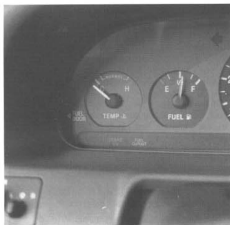
Fig. 3-1. Engine Cold/Warm-Up strategy depends on engine temperature.
