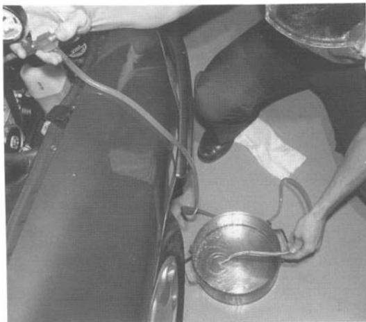
Fig. 2-4. Check return flow from regulator. Fuel-pressure gauge fitted to Schrader valve has drain valve.
