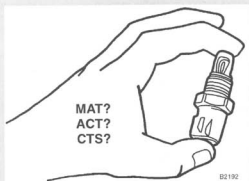
Fig. 1-4. Nomenclature can be a problem. Even within one company, Ford has different names for the same part. The name can change depending on where the engine-control system is engineered, Ford or Mazda, and even on the model year for the same engine.
