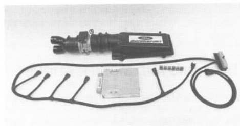
Fig. 6-1. MAF kit for F-series truck includes jumper wire harness to convert gang (bank) injection to sequential (SFI), and new EEC-IV control unit. Not street-legal in California as we go to press.
