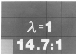
Fig. 2-5. For a warm engine, running on gasoline at part throttle, the ideal or "stoichiometric" air-fuel ratio—when there is just enough air to burn all the fuel—is 14.7:1.
