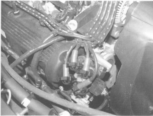
Fig. 3-14. Coil pack on each cylinder bank of 4.6L V-8 shows plug wires crossing to other bank, necessary to fire cylinders in proper pairs.
