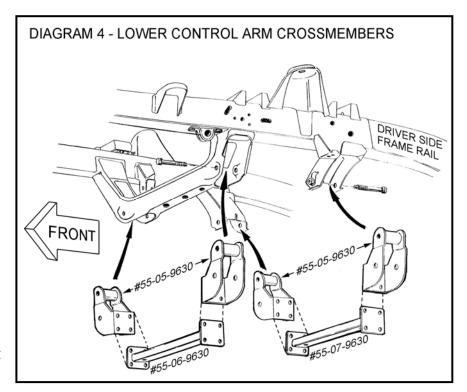
nuts pointing rearward; hand tighten only. They are tightened in a later step when the suspension is supporting the vehicle's weight.
