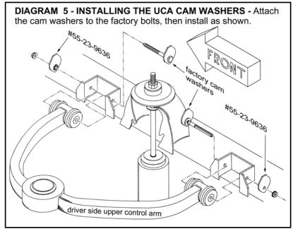
Index the "23" cam washers on the factory bolts as shown with the bung *facing* the factory frame mounts. In other words, the flat side of each washer should face the nut. Reinstall the nut and tighten the cam bolts (83-113).
