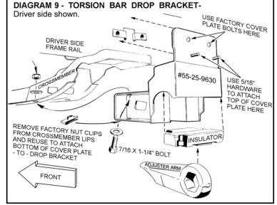
shown. Where the bracket mates to the outboard face of the frame rail, use two of the factory bolts that were originally used on the adjuster arm cover plate (35-46). Use new 7/16" hardware where the "25" bracket mates to the crossmember (37).
