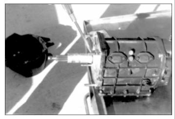
Snout will need to be cut off. The snout is only found on early model transmissions.
