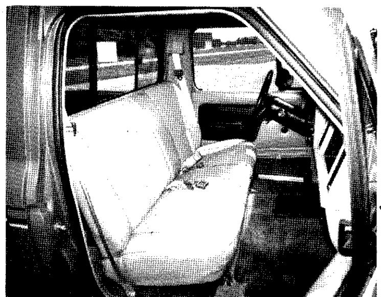
Standard bench seat has 5½-inches of travel and features 4-inch foam on Flex-O-Lator suspension w/helical springs.
