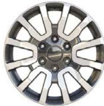
18" Machined Aluminum w/Magnetic Pockets (Opt. on XLT (302A) and Lariat (501A) w/Sport Appearance Pkg. (76E)) – 64J
