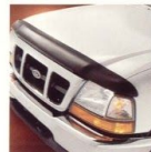
Front end cover shields the Ranger front end from stones and other road debris.
