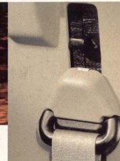
Shoulder belts have D-ring height adjusters to satisfy the comfort needs of short and tall people alike.
