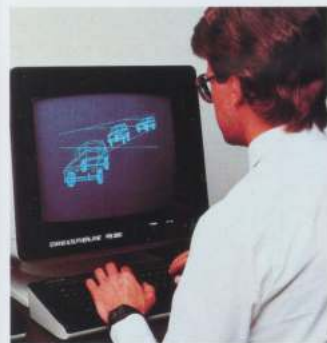
Total Vehicle Simulation helped greatly in the design of the Bronco II. Shown here is a simulated lane-changing maneuver.
