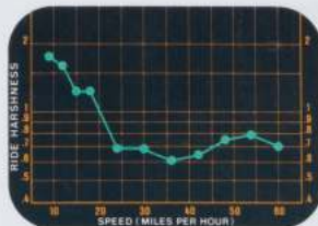
This computer plot quantifies ride quality characteristics to design engineers by analyzing vertical forces on the driver and occupants at various speeds over rough road surfaces.
