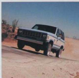
Power Hop Hill tests the ability of Bronco II's drive train components to withstand severe shock loading at Ford's Arizona Proving Ground.
