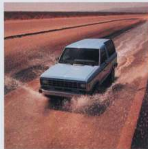
Ford's extensive corrosion testing includes a salt bath, which exposes all areas of Bronco II's underbody and engine compartment to corrosive spray.
