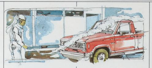
principally on making this small vehicle look as tough as the jobs it is going to perform. The aerodynamic engineers concentrated on smoothing every surface to optimize air-flow over, around and through the vehicle. The objective was to minimize wind resistance, or drag, which is critical to fuel economy goals. The more wind resistance, the more energy it takes to move the vehicle through the air.
