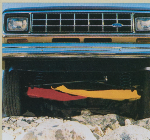
Twin-I-Beam Front Suspension (4x2)
