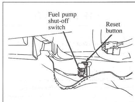
The shut-off switch is located under the dashboard to the right of the transmission hump and under the carpet. You have to pull back the carpet in order to see the shut-off switch.
