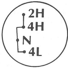
4-wheel drive operation (4H or 4L) on dry pavement is not recommended. Operating the vehicle in 4-wheel drive on dry pavement will increase tire wear, decrease fuel economy, and make 4-wheel drive disengagement difficult for the transfer case.
