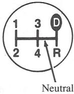
A safety feature prevents accidental shifting from **D** to R. Put the selector lever in Neutral and wait at least 3 seconds before shifting into R (Reverse) to prevent a “grinding” noise. Do not release the clutch.
