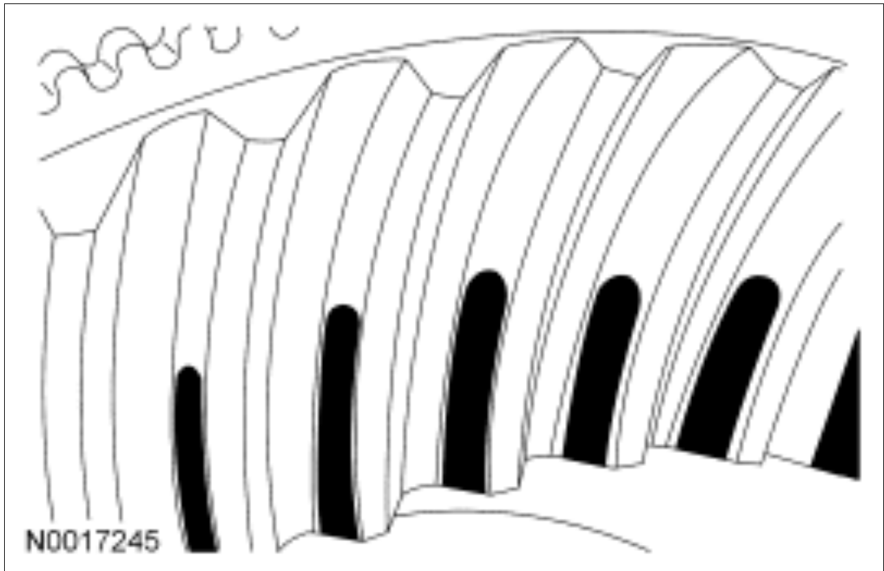
Fig 180: Identifying Tooth Contact Pattern (Thick Contact Pattern - Toe)
