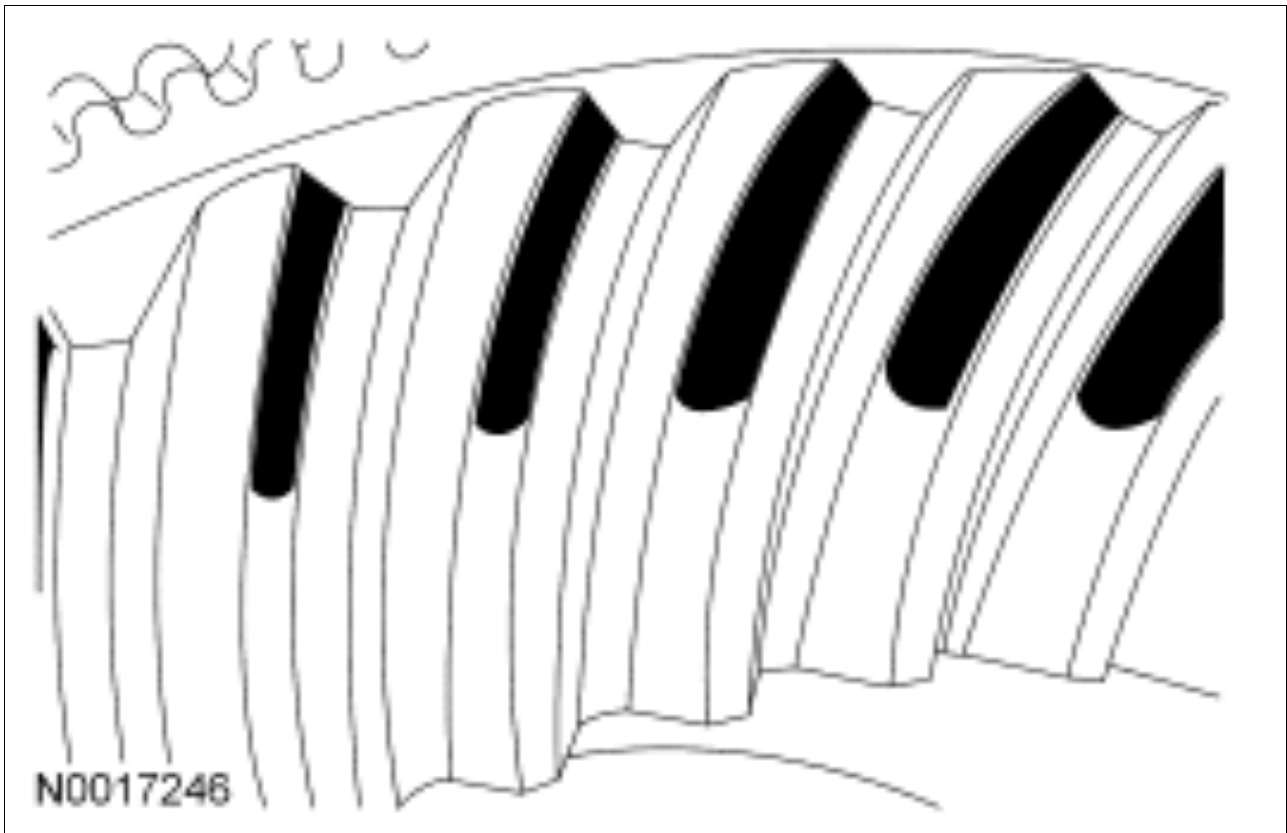
Fig 179: Identifying Thick Tooth Contact Pattern (Contacting Tooth Toward Heel)
