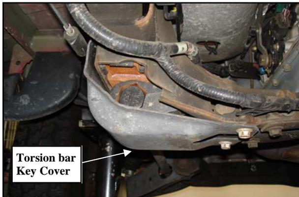
5. Measure the torsion bar adjusting screw depths and record this dimensions for later use on reassembly. Mark the orientation of the torsion bar in relation to the front A-arm.
