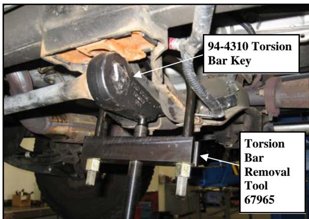
11. Install the previously removed OE bolt to the keeper, and reset the torsion bar preload bolts using the
