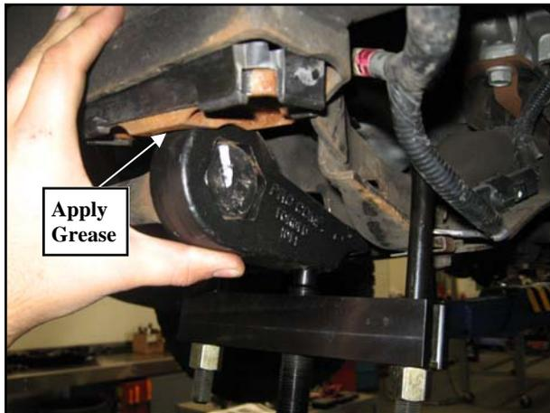
**IMPORTANT!** Make sure Torsion Bar is extended at least 1/4" inch through the Torsion Key.
