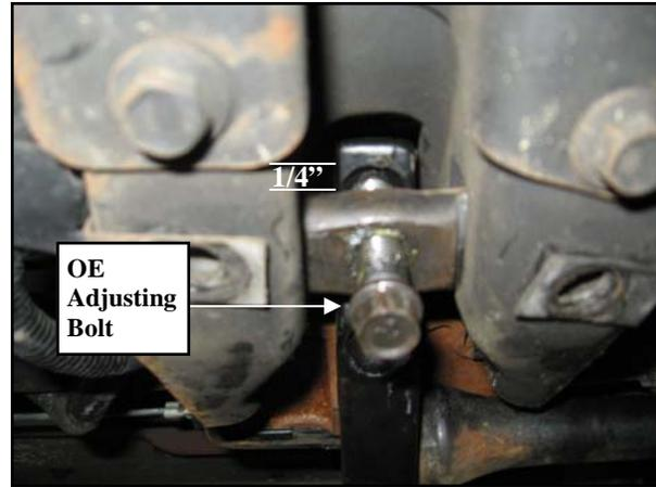
**IMPORTANT!:** Be sure that at least 1/4" of bolt threads extend beyond torsion key keeper.
