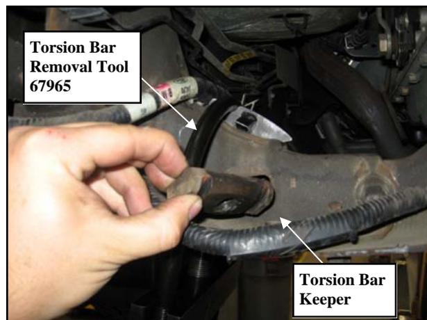
8. With the bar unloaded, slide it forward out of the OE torsion bar key and remove the key from the vehicle.
