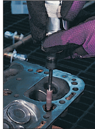
Most heads will have a lot of casting flash in the water crossovers. Use a small cartridge roll to remove that flash.
