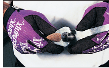
Tool changing is the first die grinder skill one learns. Most die grinders use the type of chuck that is tightened with two open-end wrenches.
